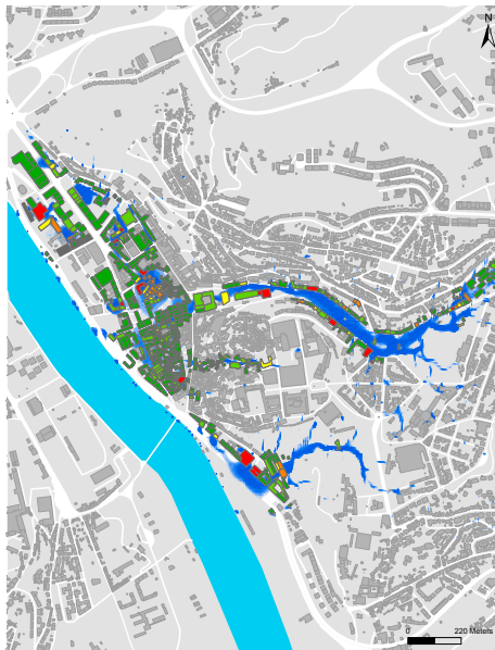
Figure 31. Flood risk - Annual average damage in buildings structure. Downtown Coimbra
